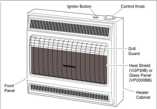
Figure 1 - Vent-Free Propane Gas Heater
